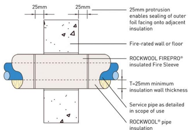
All joints to be taped with self-adhesive foil tape, including the joints where the insulated fire sleeve butts to existing insulation. To maintain the fire rating stated above, the minimum allowable length of sleeve is 50 mm. Insulated Fire Sleeves can accommodate irregularities in the division opening and the pipe O.D. up to 15 mm. Multiple pipe penetrations can be accommodated in conjunction with intumescent coated batts.
