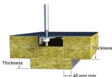
Joint Option B - Protection using 'T' section
